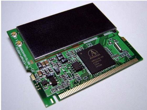
**Picture 30: Mini PCI Wireless interface card**
